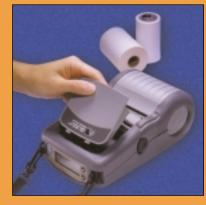
Remove and replace wireless modules on the OL 320 quickly and easily for added flexibility and capabilities, such as Bluetooth or RF LAN connectivity.
